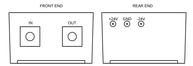
The input and output SMA connectors are located on the front end of the module, as shown above. The +24V, -24V, and GND input solder terminals are located on the opposite end.
